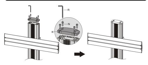
Attach the top cover to the column using the appropriate screws. Tighten all screws with an Allen key.
