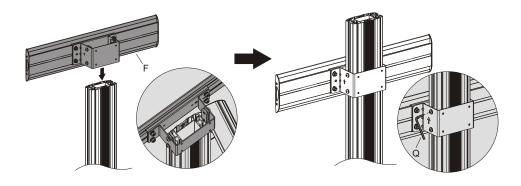
Insert the universal plate to the desired position along the column rails. Tighten all screws to secure it with an Allen key.
