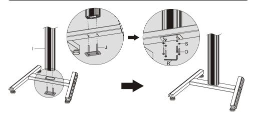
Attach the column to the assembled base using the connecting piece, secure them with the appropriate screws.
