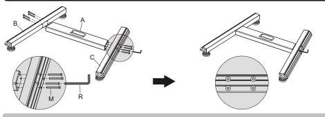
Attach the left and right base to the middle base using the appropriate screws. Tighten all screws with an Allen key.
