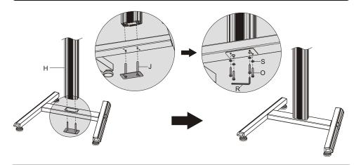
Attach the column to the assembled base using the connecting piece, secure them with the appropriate screws.
