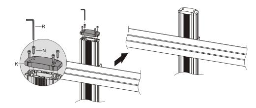
Attach the top cover to the column using the appropriate screws. Tighten all screws with an Allen key.
