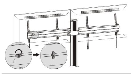
Insert the cable clamps horizontally into the plate slots, then turn the cable clamps to the vertical to secure them.
