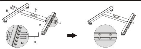
Attach the left and right base to the middle base using the appropriate screws. Tighten all screws with an Allen key.
