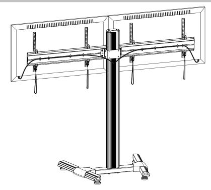
Run the cables through the cable clamps and the rubber strip.
