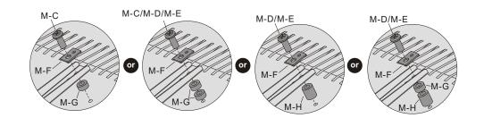
Note: Choose the appropriate screws, washers and spacers (if necessary) according to the type of screens.
