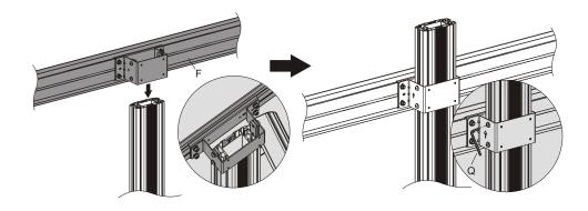
Insert the universal plate to the desired position along the column rails. Tighten all screws to secure it with an Allen key. NOTE: With the arrow pointing upward.
