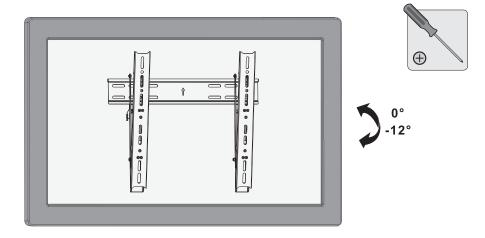
Pull from top of display to obtain the desired angle.
