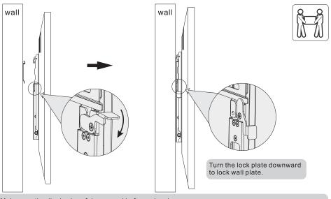
Make sure the display is safely secured before releasing.
