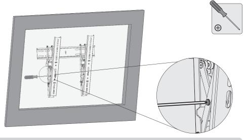
Tighten screws till display angle can be fixed.
